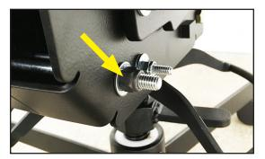
3) Using both 9/16" wrenches, remove the tilt-lock nut and washer, then slide the tilt-lock bolt all the way out of the tilt mechanism: **CAUTION - Hold the seat while removing the tilt-lock bolt to prevent sudden backward tilting.**
