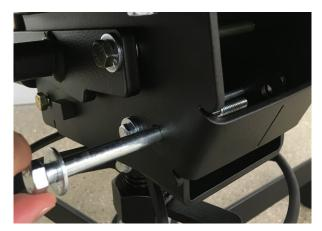
5) Replace the washer and tilt-lock nut on the end of the tilt-lock bolt. Using both 9/16" wrenches, securely tighten the tilt-lock nut onto the tilt-lock bolt:
