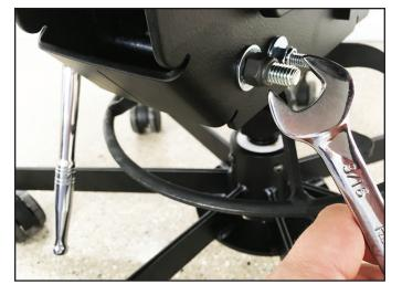
6) Using one 9/16" wrench, tighten the two hex-head bolts that were loosened in Step 1.
