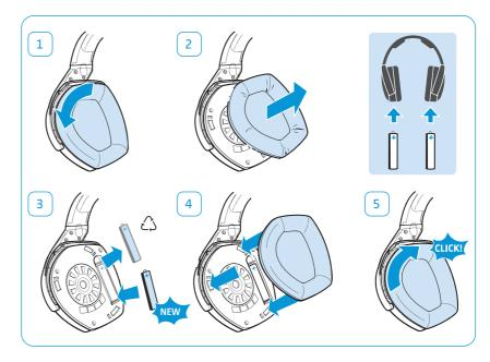
You can also power the headphones using standard batteries (AAA size, 1.5 V). Note, however, that standard batteries are not rechargeable, and if you are using standard batteries, do not place the headphones on the transmitter's headphone holder.
