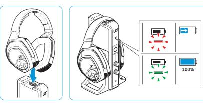
When not in use, place the headphones on the headphone holder to ensure that they are fully charged when needed. The intelligent battery charging technology prevents overcharging. When you remove the headphones from the headphone holder, the Charge status LED on the transmitter indicates the approximate operating time of the headphones (see page 10).
