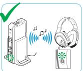
If the headphones are outside the transmission range or if there is no audio signal received from the transmitter for more than 5 minutes, the headphones switch off automatically.
