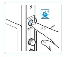
▶ Press the MODE/LEVEL button on the transmitter for 2 seconds until the *Personal Hearing* LEDs indicate the desired function.
