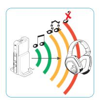
The range of the transmitter largely depends on environmental conditions such as wall thickness, wall composition etc. If you, and therefore the headphones, leave the transmission range of the transmitter, the sound drops out occasionally at first before the connection breaks down completely.
