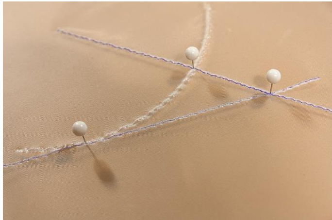
Pins are used to position a drawing tool, or to mark a certain point on a line
