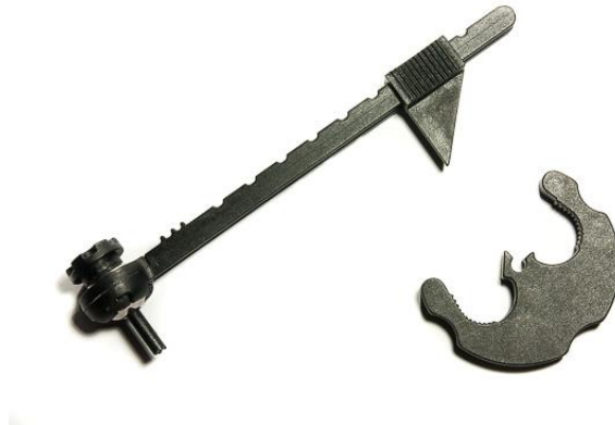
The two parts of the compass: the magnetic base and the arm
