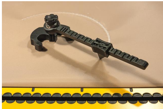
The base keeps the compass in place on the drawing surface
