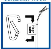
Insert the hook through the tab on the case.
