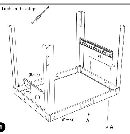
Take top shelf of metal cart and lay on side. Collect parts: FL, FR and A. Align brackets wit
