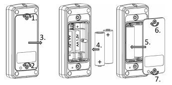
Always make sure that the seal of the battery lid is undamaged and free from debris before the lid is put back in place. Instruct the user on how to use the product in a safe way.
