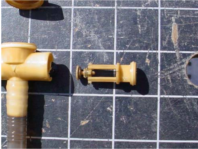
Pick-up screen and venturi system used to open the flapper valve in the bottom of the sender and draw more fuel into the assembly.
