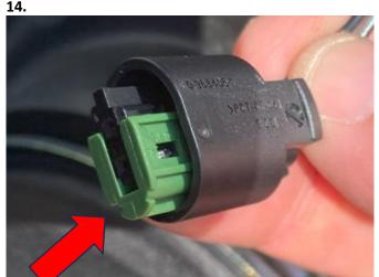
Once factory terminals are inserted into 2 position female housing, slide green lock over terminals to secure them in place.
