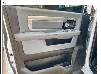
Pull out and up on the door panel, guide the manual door lock rod through the hole in the door panel as you remove it. Place the door panel off to the side while you work on installing your new harness.
