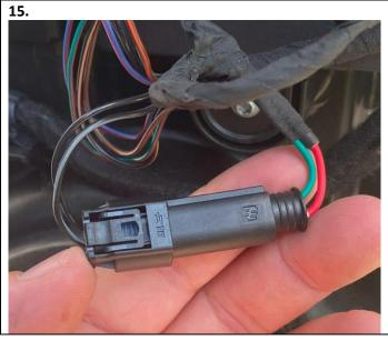
Connect the 2 position housings together. You should here a click indicating a positive engagement between both connectors.
