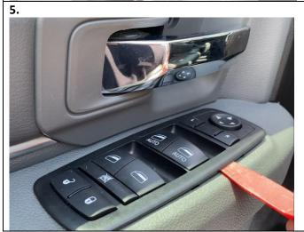
Utilizing a trim panel removal tool, gently pry the window switch module up and out of position in the door and disconnect it.
