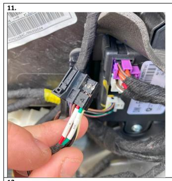
Insert supplied running light harness terminals into connector C2 at terminal position 9 and 10. Refer to terminal labels on each wire for appropriate position. Insert new terminals until you feel them click or hear an audible click indicating they are securely locked in place.
