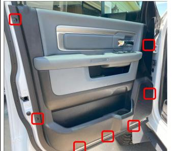
Remove push pin fasteners from around the Driver-side door panel
