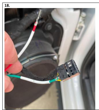
Remove existing terminals from positions 9 and 3 from housing and replace with appropriately labeled running light harness terminals into positions 9 and 3 on connector C5.
