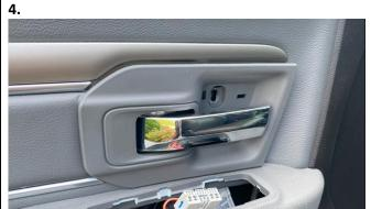
Remove door handle bezel by pulling it out towards you slightly and then towards the door hinge.
