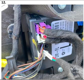
Re-assemble connector C2 and plug it back into the driver side door module.
