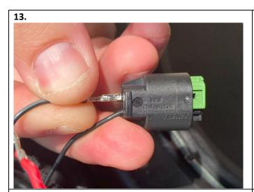
Locate the supplied 2 position female terminal housing. Pin factory wires from terminal positions 9 and 10 into the 2 position housing at position 1 and 2.
