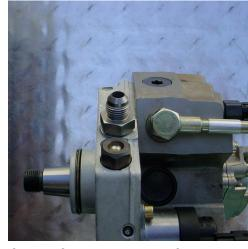
25) At this point we recommend purging the system of air before making the final connection to the injection pump.
