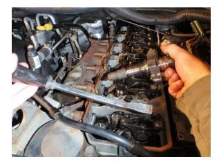
**CAUTION: DO NOT** unscrew the top electrical portion of the injector. You will not be able to reassemble it and will render the injector useless.
