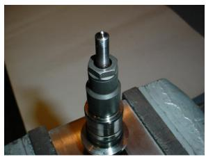
18) Note the groove in the rocker seat next to the injector hole. This is where the round end of the injector clamp will go. Remember, the injector can only go into the clamp one way.
