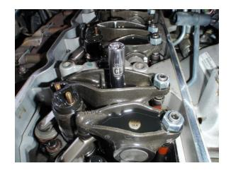
7) There are 2 parts, the rocker assembly and the bridge. Do not drop the bridge. The rocker shaft will not come out of the rocker arm as long as the bolt is left in place.
