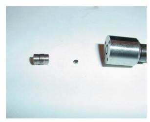
**NOTE:** We cannot stress strongly enough the importance of **NOT** losing this small puck. Replacements are not available and, if lost, you will need to replace the entire injector assembly. **DO NOT**, under any circumstances, install an injector without this puck in place. You will experience a run-away condition and engine damage **will** occur.
