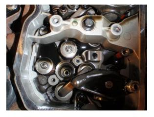
Pay attention to the round and square collar ends on the injector clamp. The round side goes next to the rocker seat. Insert the injector and clamp into the port. Place a rag over the top of the injector and use some pressure to "pop" the injector down into its seat. You will hear and feel a "click" when it seats.
