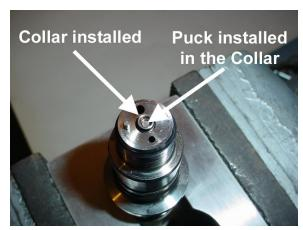
17) After the collar and "puck" have been installed place the tip back onto the injector. Screw the injector tip retaining collar back on. Torque the retaining nut/collar to 50 ft. lbs.
