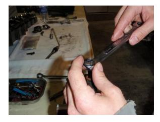
13) Unscrew the injector tip retaining nut only when you are working over a clean work surface. This photo shows the collar removed and the injector tip resting on the injector body. This is where the possibility of losing small parts becomes critical!!!
