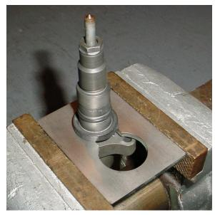
12) Using a 15 MM wrench loosen the injector tip retaining nut. These are torque to 50 ft/lbs and may require some force to break loose.
