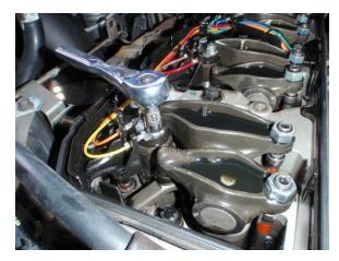
6) Using a 10 MM socket, remove the exhaust rocker arm.
