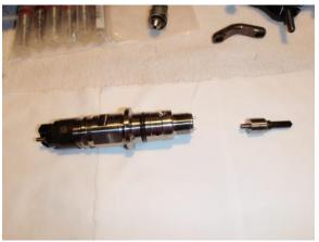
15) Stock injector tip, collar, and the **very small** "puck" (shown center) that is placed inside the injector tip collar.
