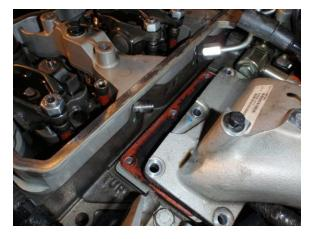
9) Using a 24MM wrench, remove the fuel connector tube that is inside the head under the fuel supply line. Connector tube is shown on the right. Simply pull to release.
