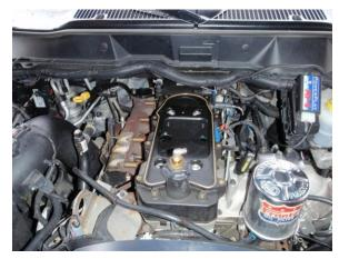
4) Remove 6 10mm valve cover retaining bolts and remove valve cover. Valve cover removed.
