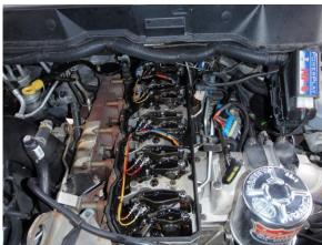
5) Using an 8MM socket remove all 12 fuel injector wiring harness nuts. Note the wire colors and their position. The nut will stay on the wire due to the crimps. These are not tight. Be <u>very</u> gentle with them. Remove the integrated injector harness assembly. Before removing, disconnect the two injector wiring harness connectors on the driver's side.
