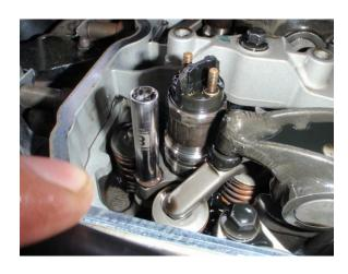
9) Remove the injector by gently rocking back and forth while pulling up. Due to carbon buildup injector may be stuck. If necessary, carefully pop the injector out using a pry bar. Make sure that the copper sealing washer comes out with the injector. If not, make absolutely sure that you remove it from the injector hole.
