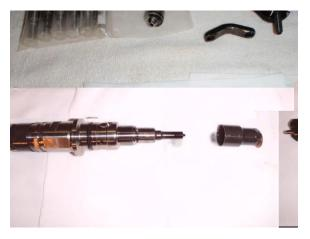
14) There are two alignment pins located in the injector face. If these fall out just place them back into the injector.
