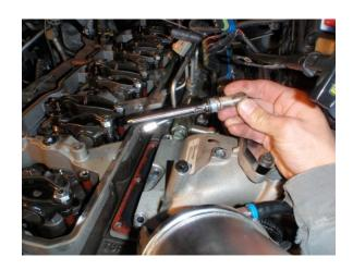
8) Using an 8MM socket, remove the 2 bolts holding down the injector clamp.
