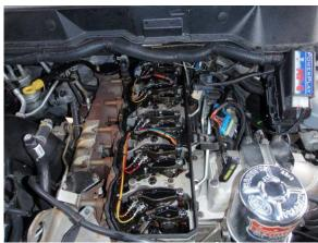
5) Using an 8MM socket remove all 12 fuel injector wiring harness nuts. Note the wire colors and their position. The nut will stay on the wire due to the crimps. These are not tight. Be **very** gentle with them. Remove the integrated injector harness assembly. Before removing, disconnect the two injector wiring harness connectors on the driver's side.
