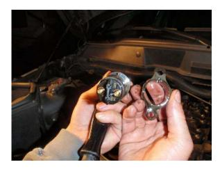
11) Place the injector in the holding tool as shown.
