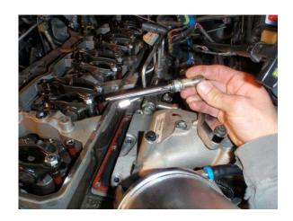
8) Using an 8MM socket, remove the 2 bolts holding down the injector clamp.
