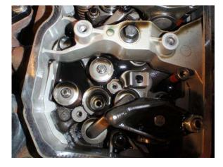
Pay attention to the round and square collar ends on the injector clamp. The round side goes next to the rocker seat. Insert the injector and clamp into the port. Place a rag over the top of the injector and use some pressure to "pop" the injector down into its seat. You will hear and feel a "click" when it seats.
