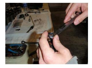
13) Unscrew the injector tip retaining nut only when you are working over a clean work surface. This photo shows the collar removed and the injector tip resting on the injector body. This is where the possibility of losing small parts becomes critical!!!
