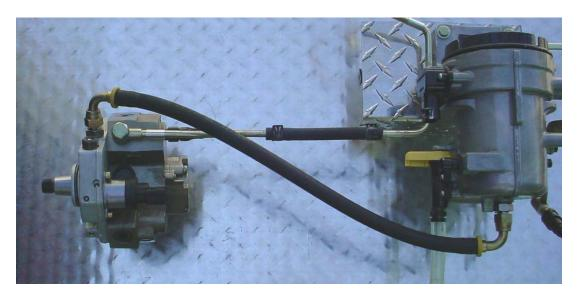
12) If access is needed for a fuel pressure sender the supplied sender tee can be installed anywhere along the new feed line. Cut the new line, install the aluminum tee and secure with the supplied clamps.
