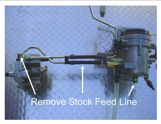
5) Completely remove the stock feed line and banjos from the bottom of the filter housing to the injection pump.
