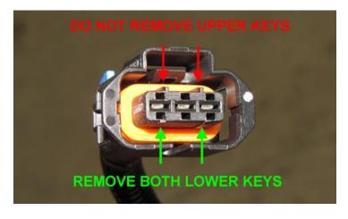
28) Using the supplied rail pressure extension harness, reconnect the rail pressure sensor at this time. Make sure connectors are fully inserted and engage the blue lock on the new rail pressure sensor connector.
