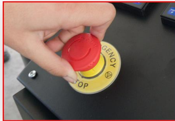
Turn it to the right (clockwise) to restart
