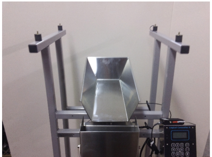
Fig. 2: Feed Pan exposed after removing Supply Hopper
