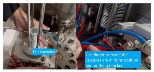
After put the capsules in the silo, use finger to move up the capsules a little to make sure the capsules are in good position and nothing blocked.
