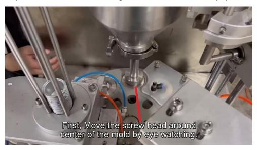
Step 2: Click Y5 filling cylinder in IO interface. It will bring up the mold and if the screw is in the center of the mold, the mold will lock the screw head. If it is not, adjust the screw position until the mold lock it.
