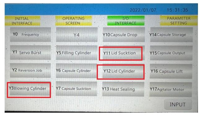
After aligning, turn on Y3 blowing cylinder, and then Y11 lid suction to suck the lid, Y12 lid cylinder to bring down the lid, then Y11 lid again to release the lid on the cup, Y12 again to bring up the sucker for the next lid.
