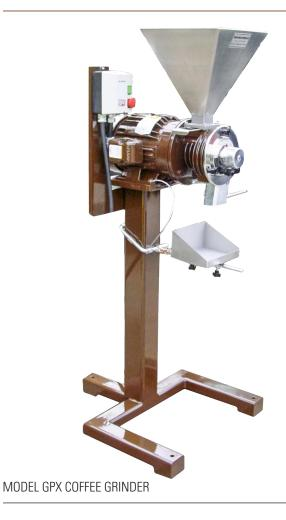
The Model GPX is an industrial disc-style grinder designed to run continuously and deliver a superior coffee grind. The GPX uses 5.5 inch diameter "diamond hard" grinding discs that are precision-cut to optimize cutting action with infinite adjustment control, resulting in a cool, uniform coffee grind for optimal brew performance.
