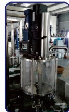
Auger Filling Controlled by Schneider Servo Motor Transparent Hopper
