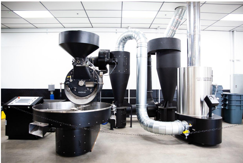
CSA-600-CAT with Probat 45 KG roaster The connection ducting shown is 10" galvanized Nordfab ducting
