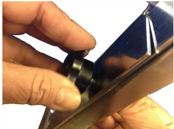
Figure 32. Tighten screw and knob on both sides under the conveyor to lock conveyor in place.
