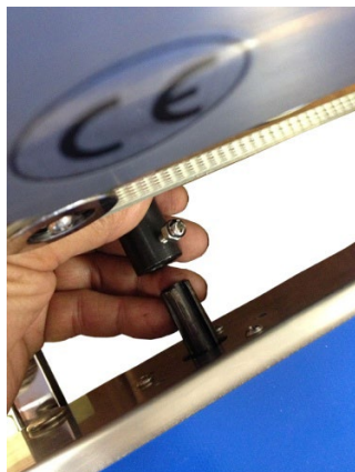
Figure 5. Insert the conveyor middle post in drive shaft. Make sure grooves are aligned.
