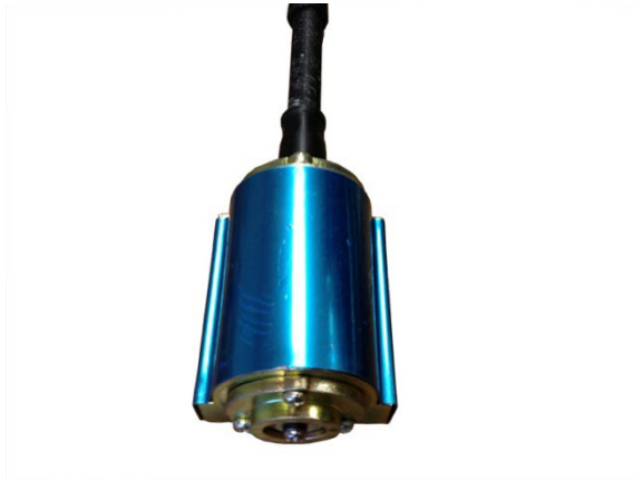
Figure 23. Remove the cover from the umbrella gear by removing the four screws on the side of the gear.
