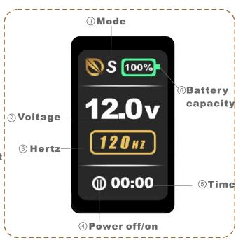
6 **Battery capacity:** Battery capacity percentage shows that if the battery is less than 5%, please charge it in time. Working time about 5-7 hours, based on operating parameters.
