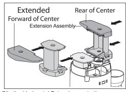
Clip the Horizontal Extensions onto the Vertical Extensions, then clip the whole extension assembly onto the Button Platforms by sliding them towards the center with the Horizontal Extensions protruding towards the front.
