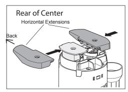
Clip the Horizontal Extensions (protruding towards the back) onto the Button Platforms by sliding them towards the center.
