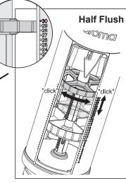
Release the Half Flush Adjusting Nut by rotating anti-clockwise ("click").
