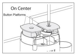
Remove cistern lid. Adjust both Button Platforms up slightly using a philips head screw driver to allow for the necessary attachments to be fitted if required.
