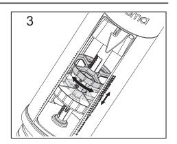
Adjust Half Flush Adjusting Nut as required (lower by 1 increment for every 3mm if the water is above the WL mark, raise if water is below WL mark). Repeat for the Full Flush in necessary.
