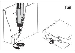
Position the Outlet Valve so the Overflow Tube is in an unobstructed position (clearing cistern walls), Firmly secure with tail nut.
