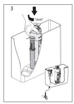
Replace Valve Cartridge and lock into Valve Base by rotating ("Click") clockwise.
