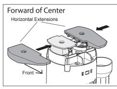
Clip the Horizontal Extensions (protruding towards the front) onto the Button Platforms by sliding them towards the center.
