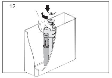
Replace Valve Cartridge and lock into Valve Base by rotating ("Click") clockwise and repeat steps 5-9 for the Half Flush.
