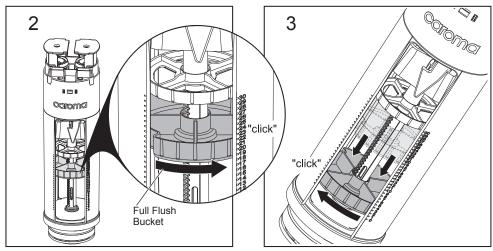
Release the Full Flush Bucket by rotating anti-clockwise ("click").
