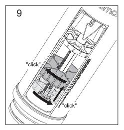
Adjust Full Flush Bucket by the difference in WL height measured.
