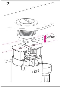
The button strikers should just contact the Button Platforms when lid is on.
