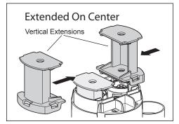
Clip the Vertical Extensions onto the Button Platforms by sliding them towards the center.
