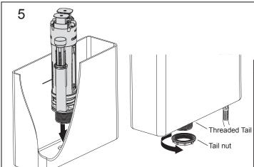
Position the Outlet Valve so the Overflow Tube is in an unobstructed position (clearing cistern walls), firmly secure with tail nut.
