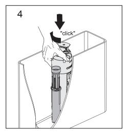
Replace Valve Cartridge and lock into Valve Base by rotating ("Click") clockwise.
