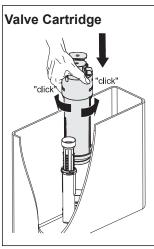
The Valve Cartridge can be detached from the base by carefully rotating it ("click") anti-clockwise and lifting.
