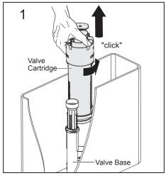
Carefully remove Valve Cartridge by rotating it ("click") anti-clockwise and lift.
