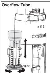
Release the Locking Clip on the Overflow Tube by rotating anti-clockwise ("click") and pull Overflow Tube upwards, exposing a series of numbers on its side.
