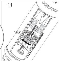
Slide down to the lowest possible setting, directly on top of the Full Flush Bucket and secure its position by rotating clockwise ("click").
