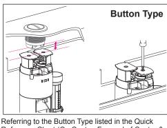
Reference Chart (On Center, Forward of Center & Rear of Center) attach the Button Caps as required and adjust each Button Platform using a philips head
