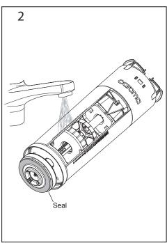
Wash seal to remove any dirt and inspect for damage. If necessary remove seal and replace (Spare Part Kit 750017).
