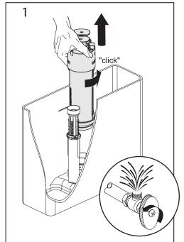
Remove lid, turn off mains water and flush cistern empty. Carefully remove Valve Cartridge by rotating it ("click") anti-clockwise and then lifting.
