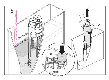
Measure the difference in height between the original Working WL and the resultant WL after refilling. Carefully remove Valve Cartridge again.
