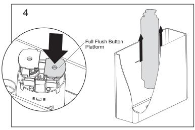
Turn off mains water, flush cistern empty and remove existing outlet valve.
