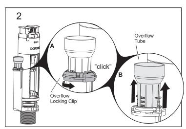
Release the Locking Clip on the Overflow Tube by rotating anti-clockwise ("click") and pull Overflow Tube upwards, exposing a series of numbers on its side.
