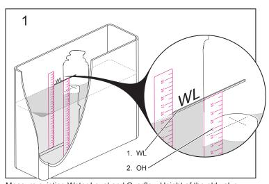
Measure existing Water Level and Overflow Height of the old valve. Set the Overflow height on the new valve to which ever is the lowest:
