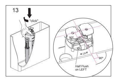
Finally, with the Half Flush Button on the left hand-side, replace Valve Cartridge and lock into Valve Base by rotating ("Click") clockwise.
