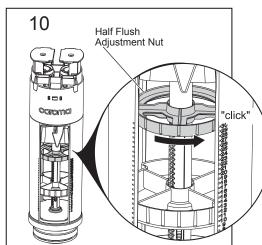
Release the Half Flush Adjusting Nut by rotating anti-clockwise ("click").
