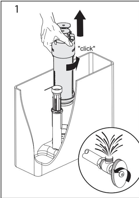
1 Remove lid, turn off mains water and flush cistern empty. Carefully remove Valve Cartridge by rotating it ("click") anti-clockwise and then lifting.
