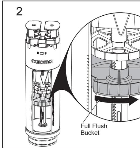
Release the Full Flush Bucket by rotating anti-clockwise ("click").
