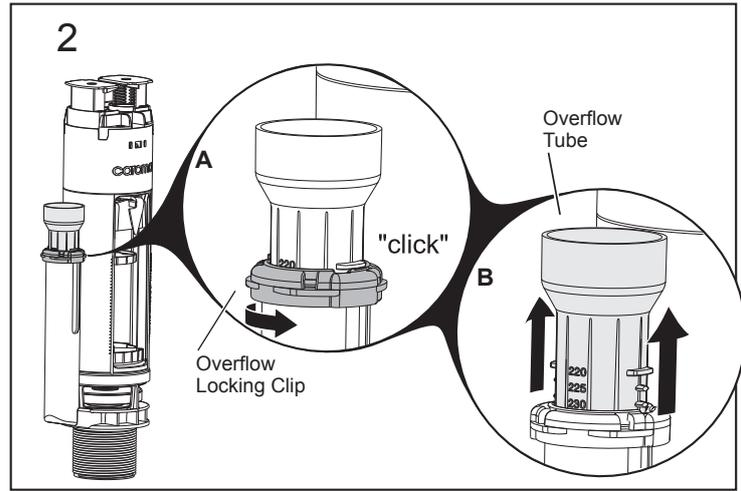
Release the Locking Clip on the Overflow Tube by rotating anti-clockwise ("click") and pull Overflow Tube upwards, exposing a series of numbers on its side.
