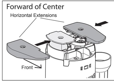
Clip the Horizontal Extensions (protruding towards the front) onto the Button Platforms by sliding them towards the center.
