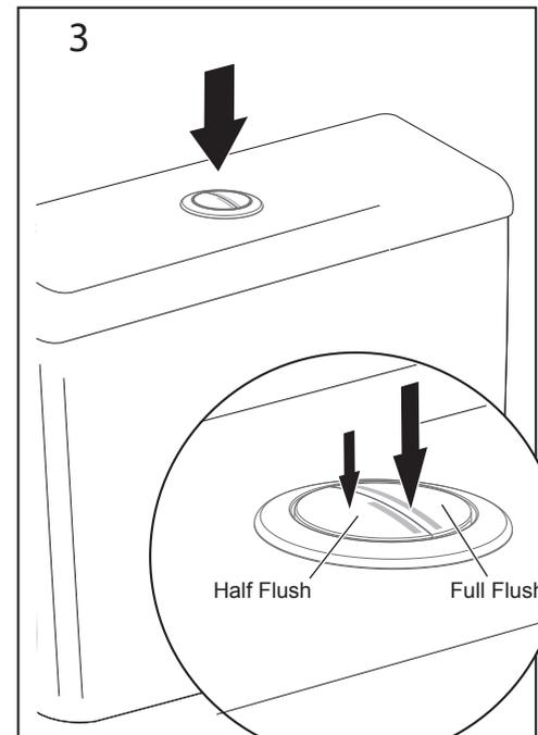
Replace lid complete with button and bezel assembly and test both buttons to ensure they activate the outlet valve.
