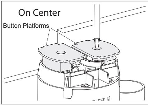
Remove cistern lid. Adjust both Button Platforms up slightly using a philips head screw driver to allow for the necessary attachments to be fitted if required.
