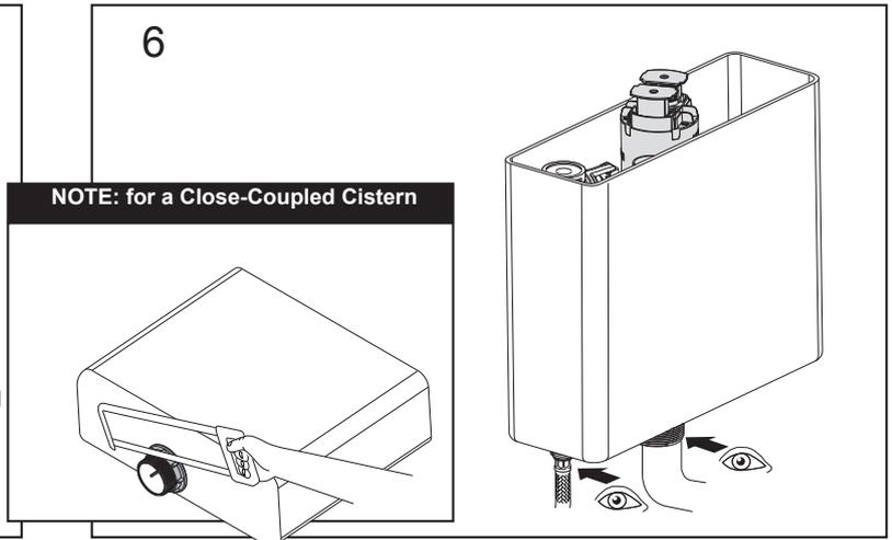
**Note:** If you have a close-coupled suite (i.e. If the cistern seals directly on top of the pan and does not have a flushpipe), carefully cut off the remainder of the Threaded Tail using the bottom edge of the tail nut as a guide.
