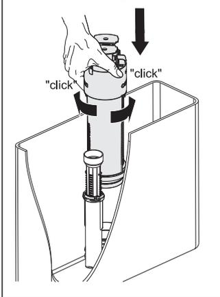
The Valve Cartridge can be detached from the base by carefully rotating it ("click") anti-clockwise and lifting.
