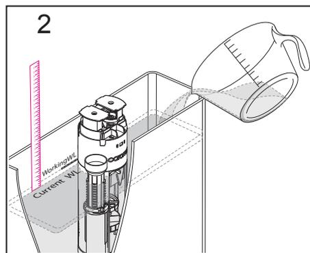
Referring to Flush Volume Chart (in step 7, pg. 4), add the required half flush volume using graduated container.
