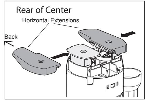
Clip the Horizontal Extensions (protruding towards the back) onto the Button Platforms by sliding them towards the center.
