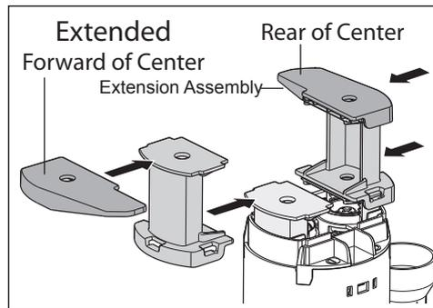
Clip the Horizontal Extensions onto the Vertical Extensions, then clip the whole extension assembly onto the Button Platforms by sliding them towards the center with the Horizontal Extensions protruding towards the front.
