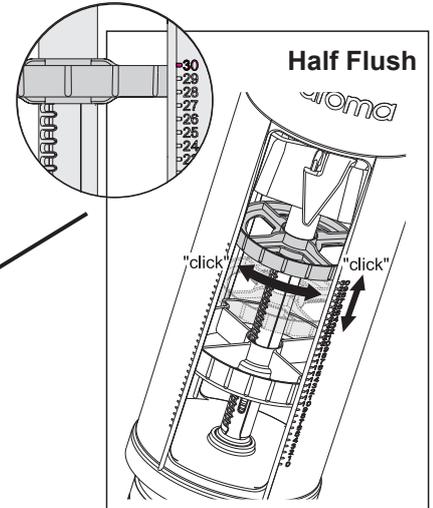
Release the Half Flush Adjusting Nut by rotating anti-clockwise ("click").
