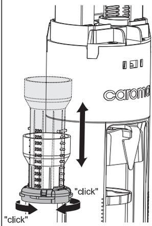
Release the Locking Clip on the Overflow Tube by rotating anti-clockwise ("click") and pull Overflow Tube upwards, exposing a series of numbers on its side.
