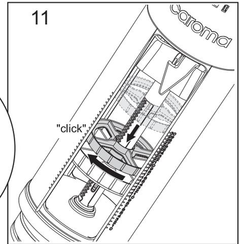
Slide down to the lowest possible setting, directly on top of the Full Flush Bucket and secure its position by rotating clockwise ("click").
