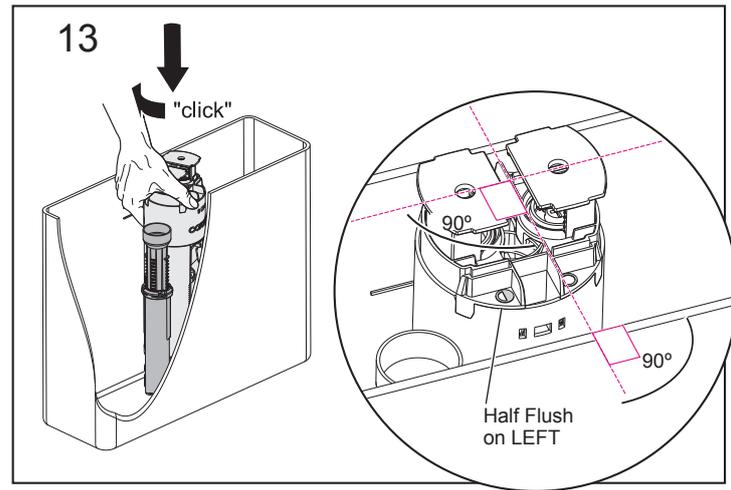
Finally, with the Half Flush Button on the left hand-side, replace Valve Cartridge and lock into Valve Base by rotating ("Click") clockwise.
