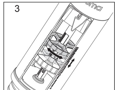
Adjust Half Flush Adjusting Nut as required (lower by 1 increment for every 3mm if the water is above the WL mark, raise if water is below WL mark). Repeat for the Full Flush in necessary.
