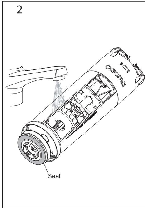
2 Wash seal to remove any dirt and inspect for damage. If necessary remove seal and replace (Spare Part Kit 750017).
