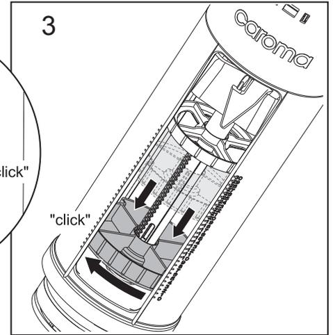
Slide down to the lowest setting and secure its position by rotating it clockwise ("click").
