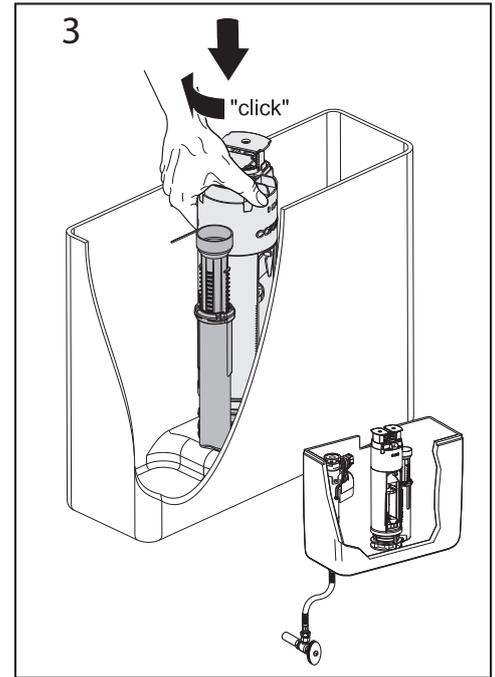
3 Replace Valve Cartridge and lock into Valve Base by rotating ("Click") clockwise.
