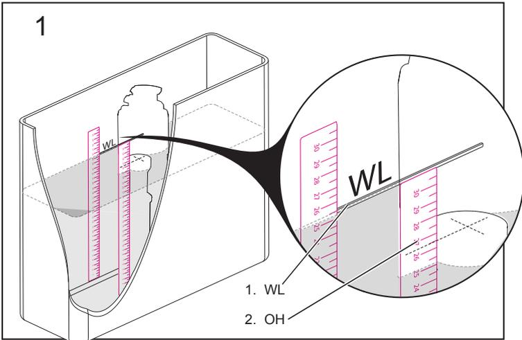
Measure existing Water Level and Overflow Height of the old valve.
