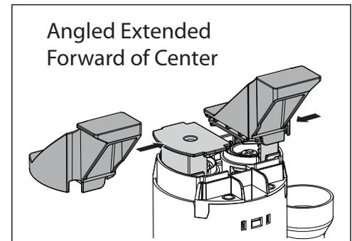
Clip the Angled Extensions (protruding towards the front) onto the Button Platforms by sliding them towards the center.
