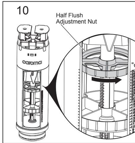
Release the Half Flush Adjusting Nut by rotating anti-clockwise ("click").
