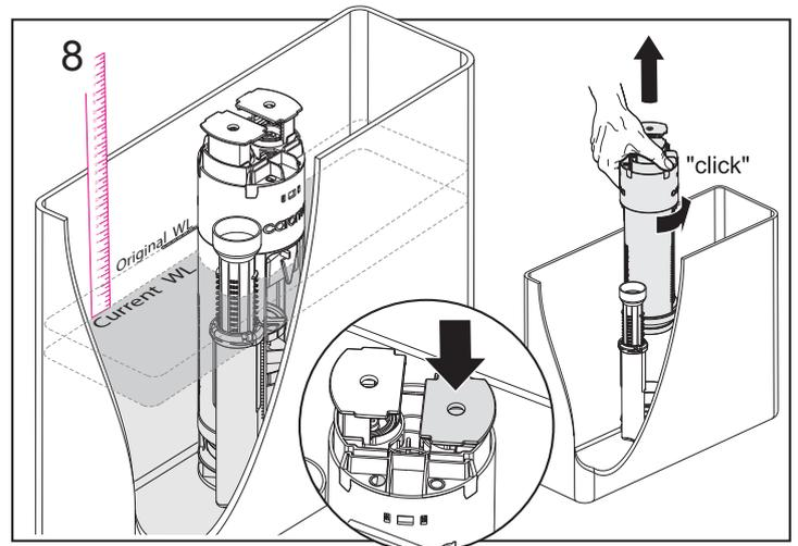
Measure the difference in height between the original Working WL and the resultant WL after refilling. Carefully remove Valve Cartridge again.
