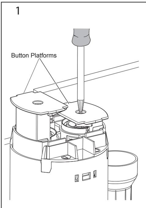
Remove cistern lid. Adjust each Button Platform using a philips head screw driver.
