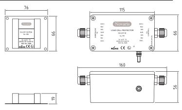
Figure 2: Dimensions of the load cell protectors
