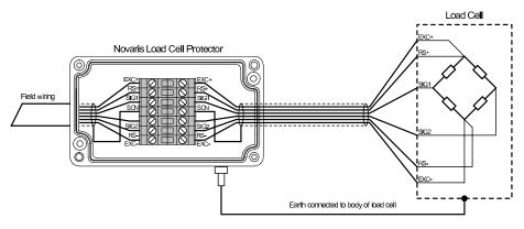
Figure 3: Installation of load cell protector
