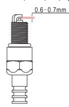
Standard Spark Plug: E6TC/E6RTC/BPR6HS
