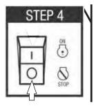
Turn the engine ON/OFF switch to the "OFF" position.
