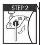
Turn the fuel valve to the "OFF" position.
