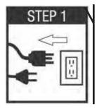
All electrical loads MUST be disconnected from generator.
