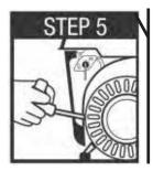
Pull the starter grip lightly until you feel resistance, then pull briskly to start the engine.
