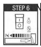
Move the choke lever to the "OPEN" position.
