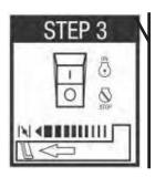
Move the Choke lever to the "CLOSED" position.
