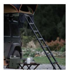
If the terrain does not allow the ladder to have a stable, even base, move your vehicle to another spot. Do NOT install the ladder on uneven ground, or on rocks, sand, or mud. Place the ladder at an approximate 70° angle as pictured below, and make sure it is firmly planted in the ground. The ladder should be able to offer support to the extension panel and the
