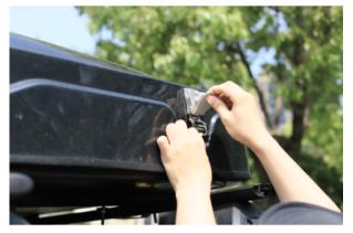
2. With one hand, push up the hard shell. The gas struts will allow it to open on its own
