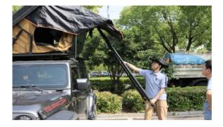
3. After the extension floor has beenlowered, securely install the ladder.
