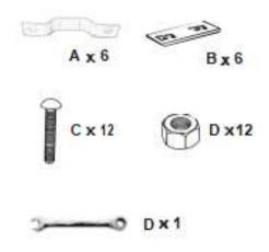
**NOTE:** apply lubricant to the bolts and nuts before tightening to reduce the risk of thread galling.
