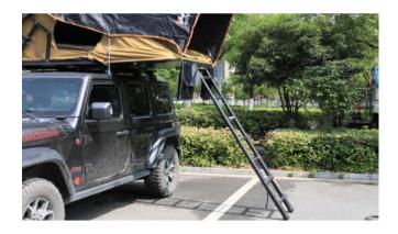
1. Pull the ladder towards you, allowing it to extend completely (NOTE: when you first use the roof tent, you will first need to undo the velcro strap on the ladder)
