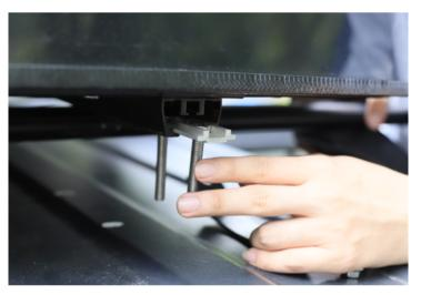
3. Have one person lift the roof tent, while another person slides the piece over the cross bar, so that one bolt is on each side of the cross bar:
