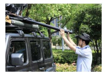
3 Reachinto the rooftent to grab the black nylon strap attached to the top of the shell. Pull down on the strap to close the hard shell:
