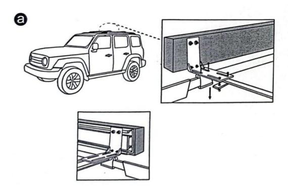
Mounts directly on the roof wishbone
