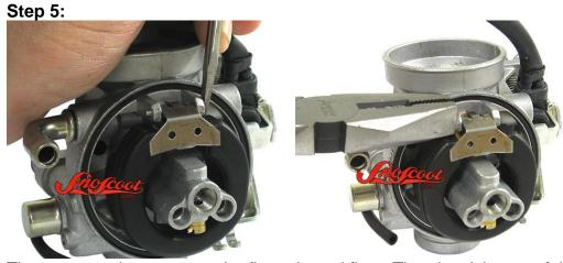
The next step is to remove the float pin and float. The pin sticks out of the mounting flanges on either end, but it is removed by pushing it to the side with a flat head screw driver (side shown in the picture above), then pull it out the rest of the way with a set of
