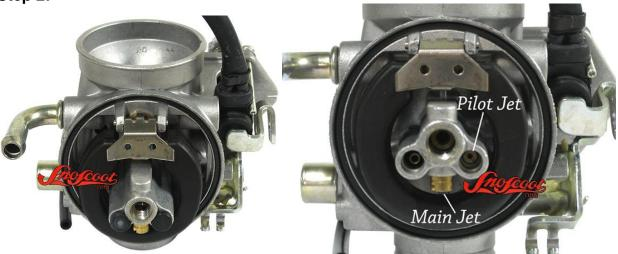
After removing the carburetor bowl, the next step is to pull out the rubber plugs, if they are present under the fuel bowl. These plugs will pry out with a flat head screw driver. Under one of the plugs, you will see your pilot jet and a long brass tube. The pilot jet and main jet are labeled on the above picture on the right.
