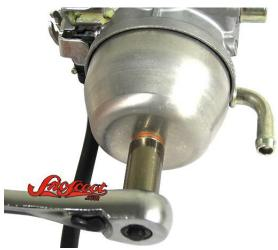
After removing the carburetor from the snowmobile, you first must remove the bowl. This operation only requires a 10 mm wrench.
