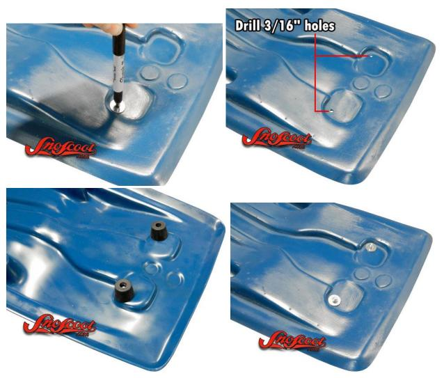
First, align a fender washer on the corner of the square bump on the bottom rear of the seat, as shown above, and make a mark with a marker. Drill the two holes shown above with a 3/16" drill bit. Next, take the included 5 mm diameter socket head cap bolts and insert them through the included rubber bumpers and then insert the bolts through the holes you drilled. On the top
