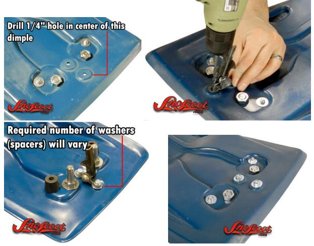
Drill a 1/4" hole in the center of the rear seat latch mounting dimple as shown above, then use your seat latch as a guide to drill the hole in the other dimple. Then bolt in the seat latch (uses included 6mm bolts) and put a few of the included fender washers between the seat pan itself and the latch. You may have to use as many as 7 of the included fender washers as spacers. On the top of the seat pan, use one two of the remaining fender washers and the included nuts as shown above.
