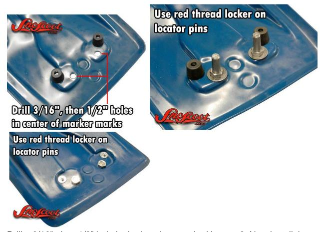
Drill a 3/16", then 1/2" hole in the locations marked in step 2. Now install the included stainless seat studs, nuts, and washers as shown above. On the bottom of the seat, you will use both a nut and washer, but on the top of the seat pan, no washer will be used. Be sure to use red thread locker on the locator pin threads and tighten the studs and nuts.
