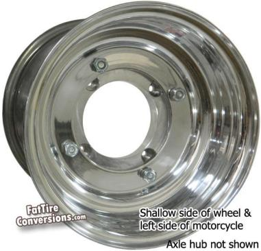
With the hub adapter bolted to the stock hub, face the deeper side of the wheel toward the newly installed wheel adapter and slide it over the hex head bolts you inserted into the hub adapter above. Now fasten the wheel to the adapter using the larger included lock washers and lock nuts. Reinstall the entire rear wheel, hub, and axle assembly onto the swingarm and you are good to go!
