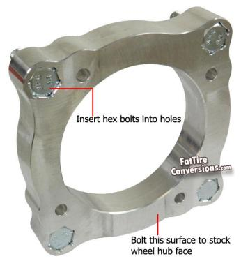
Next, insert the included bolts into the bolt holes as shown above and slide the assembly over the stock wheel studs. Use the smaller lock washers and lock nuts to fasten the aluminum hub adapter/spacer to the stock rear wheel axle hub. A deep socket will be required to tighten the nuts.
