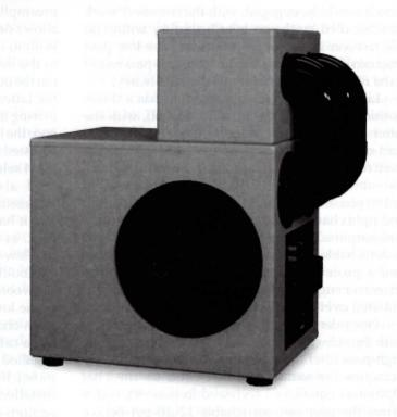
a weight of 93 pounds. Second, the dual, rearmounted 3-inch ports have been replaced by dual, rear-mounted 4-inch jobs that extend into the enclosure and then curve downward towards the bottom. With each being over two feet long, they allow the system to plumb the low-bass range strongly and play loudly, and do so without the port wind noise that was sometimes audible with the earlier versions.
