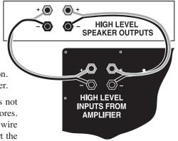
Run the wires from your system's amplifier to the subwoofer's HIGH LEVEL INPUTS. For each channel, run wire from the red (+) outputs on the amplifier to the subwoofer's red (+) inputs, and from the black (-) outputs on the amplifier to the subwoofer's black (-) inputs. Make sure the black amplifier outputs are "true ground." Bridged outputs cannot be used.
