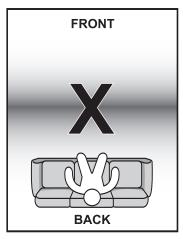
Avoid placing the subwoofer halfway between the front and back walls. Avoid sitting there as well.
