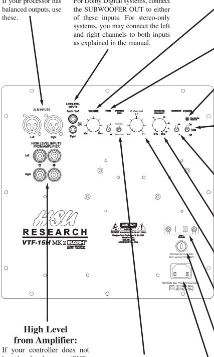
have low level outputs (SUB-WOOFER, LFE, or fullrange preamp outputs), use these color coded connectors. Run speaker wire from your amplifier or receiver's speaker terminals to tap the signal.
