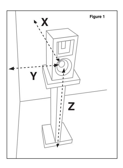
If the HB-1  $\mbox{mk2}$  is used as a center channel, it's best to use it in the normal upright position just like the left and right speakers. You can also lay it on its side at the expense of horizontal polar response.
