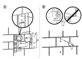
Caution: The minimum depth of the concrete must be 8". Do not drill pilot holes into the mortar between the concrete.
