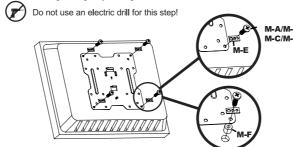
1 Level the wall plate and make 3 marks with pencil to show where to drill the pilot holes.
