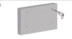
Caution: The minimum depth of the concrete must be 8". Do not drill pilot holes into the mortar between the concrete. SUNCRAFT SOLUTIONS INC. LIMITED WARRANTY
