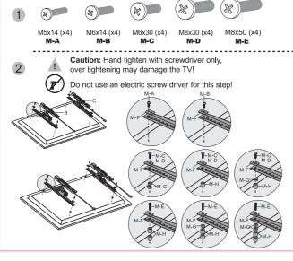
Step 3: Install Wall Plate on Concrete
