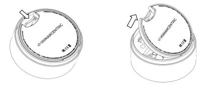
**2.** Remove old batteries if replacing them, and place fresh batteries in the proper orientation according to markings in the battery pockets.
