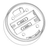
**3.** Slide the battery cover under the ledge and push the cover tab back in until you hear a click.
