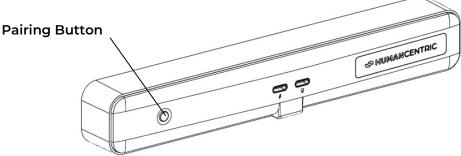
**3.** Press the power button once to wake up the controller and turn on any existing lights already paired to the controller. Then hold the power button for about 5 seconds until both indicator lights flash and then release immediately. The controller will enter into pairing mode and the indicator lights will alternate lighting up.
