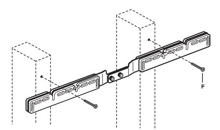
**WARNING:** Do not over tighten the screws. Over tightening will cause the end of the bracket to move away from the wall.
