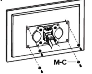
Note: Use the screws included with your mount to complete this step. If necessary, use the included washers to achieve the correct fit.
