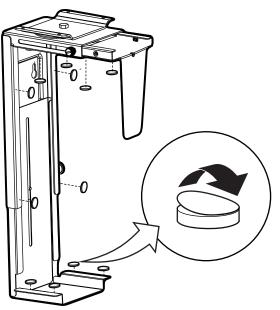
Apply the 12 felt pads to the mount in the positions shown below.
