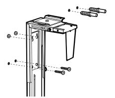
Hang the mount on the top two screws. Then tighten all four screws to secure the mount in place.
