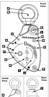
Ù R 8 S-Front View - A. Swivel top, B. Swivel Axle, C. Sideplate, D. Rope path for lower friction, E. Rope path for higher friction, F. Pivoting Bollard Axle, G. Product branding, H. Ratings for Minimum Breaking Strength (MBS), and Working Load Limit (WLL), I. Rope size, J. Rope path toward load, K. Sideplate release button, L. Button must be fully extended and locked, M. Manufacturer, N. Country of manufacture, O.
