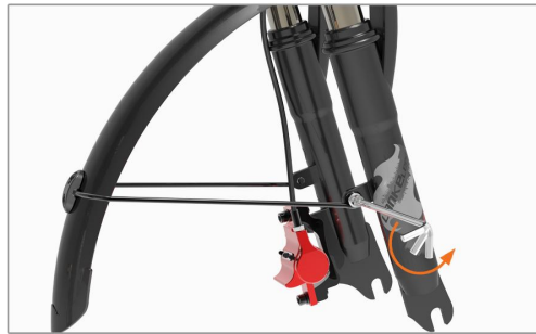
02 Fix the branches of the mudguard in the correct position and tighten the screws
