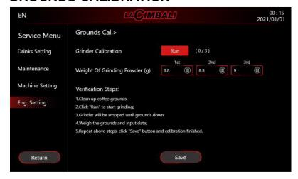
When using different coffee beans, the amount of powder may deviate from the factory calibration standard. Therefore, it is recommended to do ground calibration with the chosen beans before using the coffee machine.
