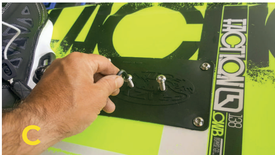
TIGHT THE SCREWS ON THE MAST
