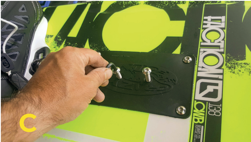
TIGHT THE SCREWS ON THE MAST
