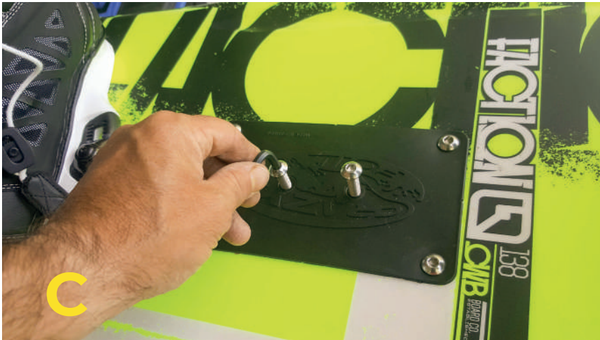
TIGHT THE SCREWS ON THE MAST
