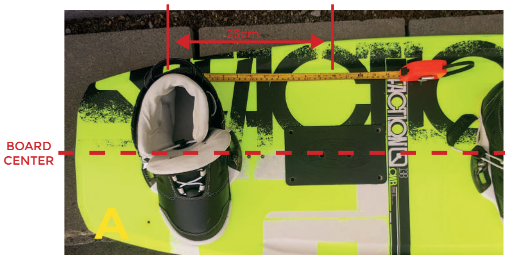
POSITION TOP PLATE ON THE BOARD, MIDDLE OF IT 25cm FROM MIDDLE OF THE REAR FOOT. PLATE CENTERED AND ALIGNED WITH THE BOARD.
